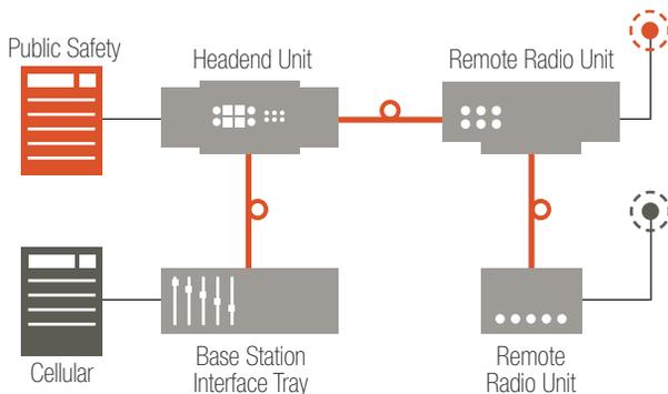
**FIGURE 3:** When designing an integrated system, the varying wavelengths from both public safety and cellular frequencies can be strategically designed to ensure that these RF signals are not competing or affecting each other negatively.
