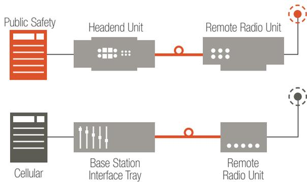
**FIGURE 2:** When these two systems are implemented separately, they should be installed in parallel if feasible. Laying cable for each system at the same time reduces ceiling and riser work.
